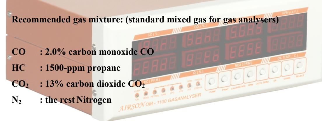
CO<sub>2</sub> should be present in the calibration gas to minimize the CO/CO<sub>2</sub> Quench effect by molecular collision processes.
